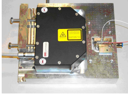
Figure 3.20: Piezo air-jet mounted in measuring frame together with the laser twin sensor.
