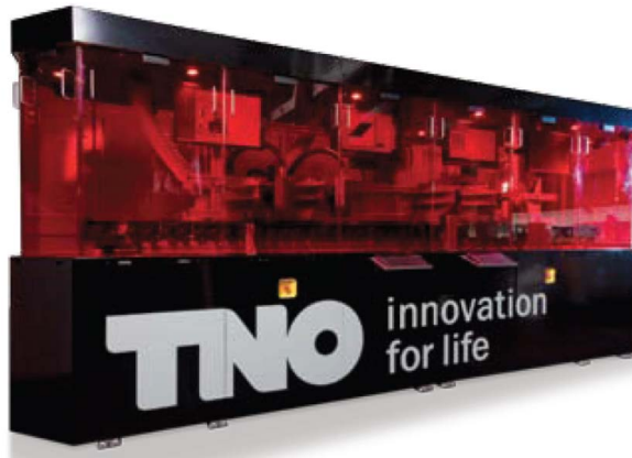
Figure 7.1: Additive manufacturing production machine. 100 carriages travel at high speed (2 m/s) past stationary deposition units. Single pass deposition units supply the passing product with a full layer with each pass. The production carriages are connected with minimum space in between to reach optimal coverage of the deposition units. No time is lost by back and forth motions since all products follow a repeating circular path. Instead of building a 50x75x6 mm part in 1.5 hours this layout provides a platform to reach a finished part every 6 seconds (100 parts in 10 minutes) [85].
