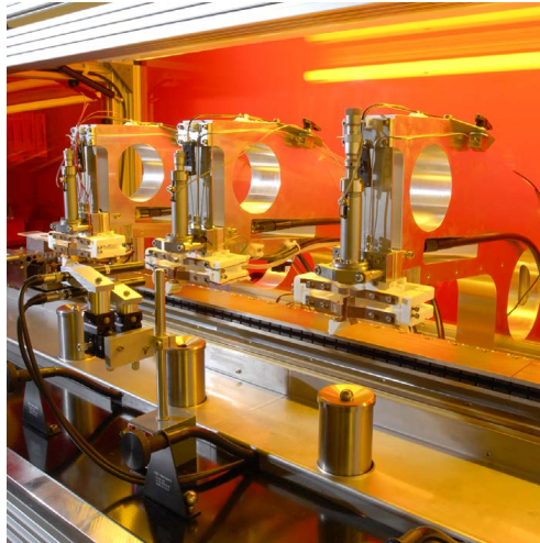
Figure 6.1: Three printheads combined in one test rig.
